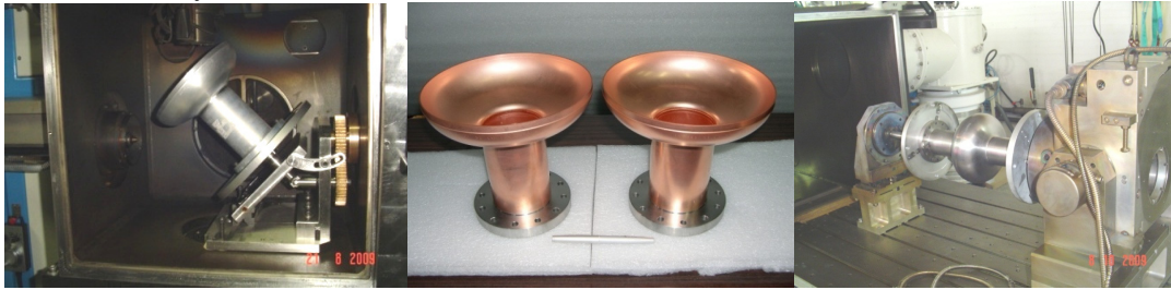
FIGURE 3. a, b & c, shows the fabrication stages of prototype Single cell Aluminum, Copper and Niobium cavities.
