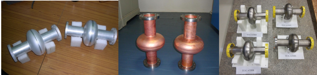
FIGURE 1. a, b & c, shows the prototype 1.3 GHz Single cell Aluminum, Copper and Niobium cavities.
