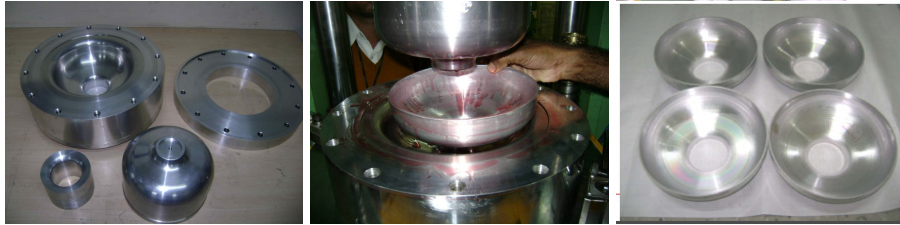
FIGURE 2. a, b & c, shows the forming tool, process & 1.3 GHz formed half cells .
