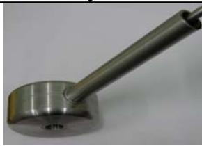
FIGURE 2. Drift tube assembly with embedded permanent magnet quadrupoles
