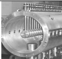
FIGURE 1. Drift tubes mounted in the DTL tank
