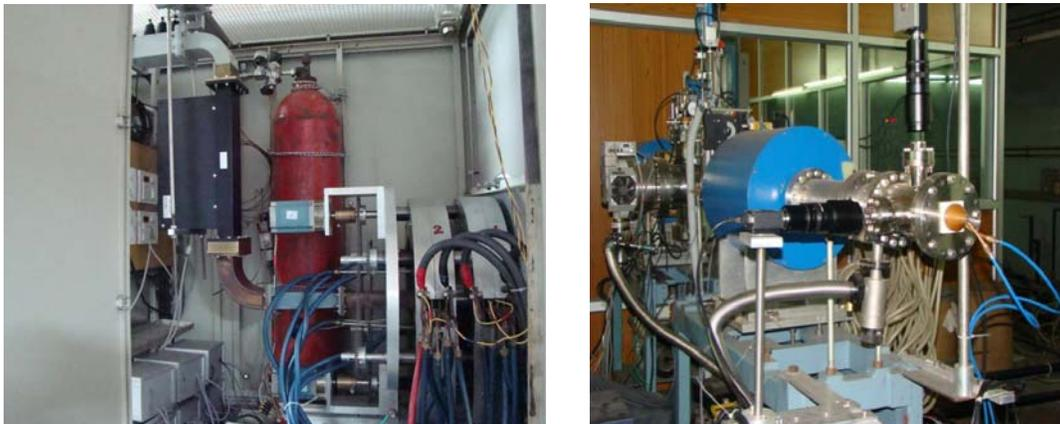
**FIGURE 1.** 2.45 GHz microwave ion source on the high voltage deck (left) and solenoid based low energy beam transport line (right).
