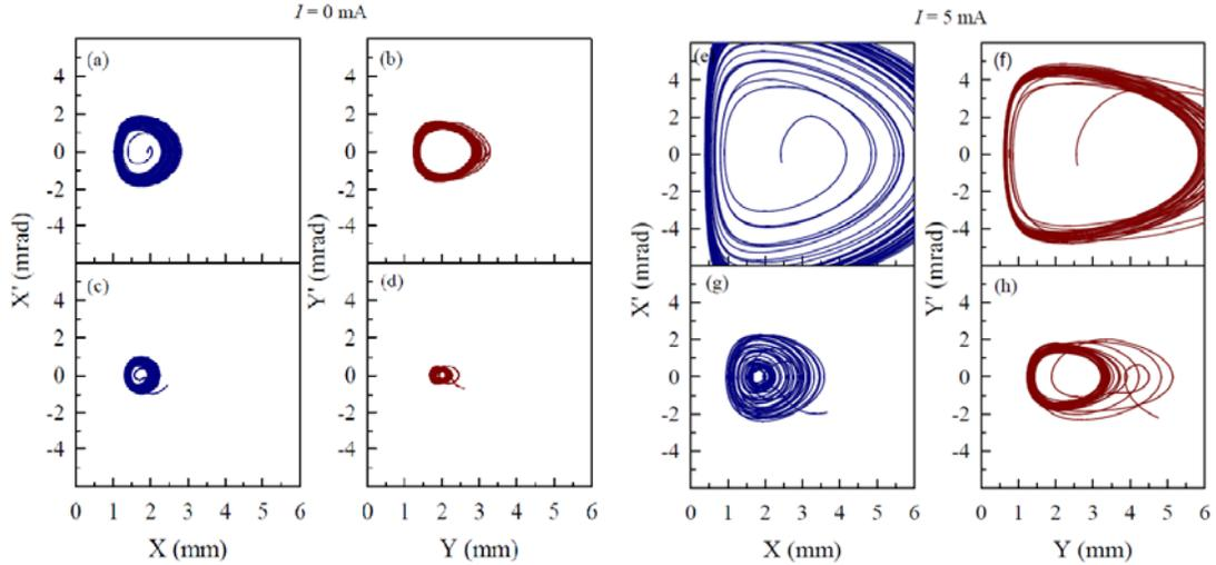
**FIGURE 2.** Plot of envelope slope with size up to final radius for  $I = 0$  mA and 5 mA for both planes. Plots 2(a) and 2(b) were obtained with matched initial beam sizes  $X_m = 1.92$  mm and  $Y_m = 3.26$  mm at the injection. Plots shown in 2(c) and 2(d) were obtained after optimization. Plots 2(e) and 2(f) are for  $I = 5$  mA with same input conditions as in 2(c) and 2(d). Optimized plots are shown in 2(g) and 2(h).
