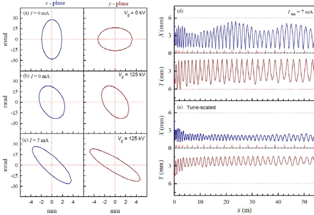
**FIGURE 3.** Input ellipses for (a) matched envelope sizes for  $I = 0$  mA, (b) optimized envelopes with acceleration and  $I = 0$  mA, (c) optimized envelopes with acceleration and  $I = 5$  mA. (d) beam envelopes up to 10 MeV with initial conditions  $X_0 = 4.9$  mm,  $X'_0 = -30$  mrad,  $Y_0 = 5.3$  mm,  $Y'_0 = -35$  mrad and (e) envelopes when betatron tunes are scaled by 1.15 times with same initial conditions as in (d).
