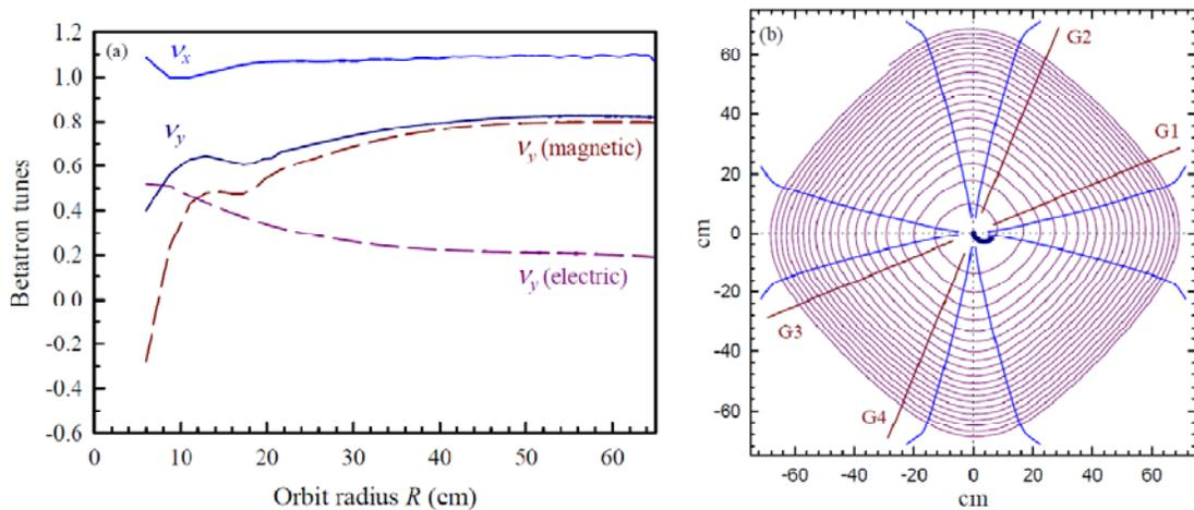
**FIGURE 1.** (a) Betatron tunes as a function of orbit radius  $R$ . (b) Position of the inflector, location of the accelerating gaps ( $V_g = 125$  kV) and accelerated orbits of proton from 80 keV to 10 MeV.
