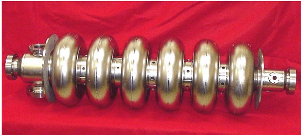
**>80% of CEBAF cavities were made with CBMM Pyrochlore ore based niobium
