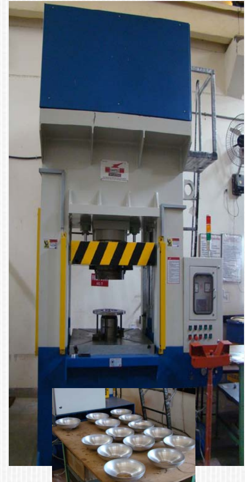
Formed Niobium Half cell
