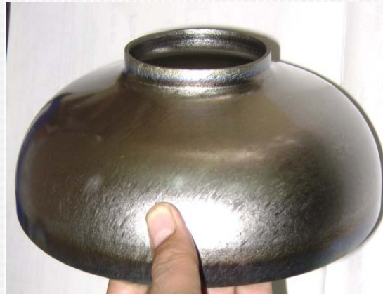
Formed Niobium Half cell
