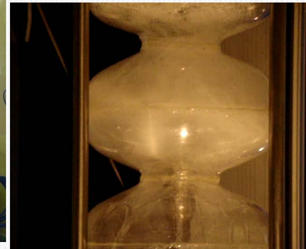
High Pressure Cleaning of dummy cavity
