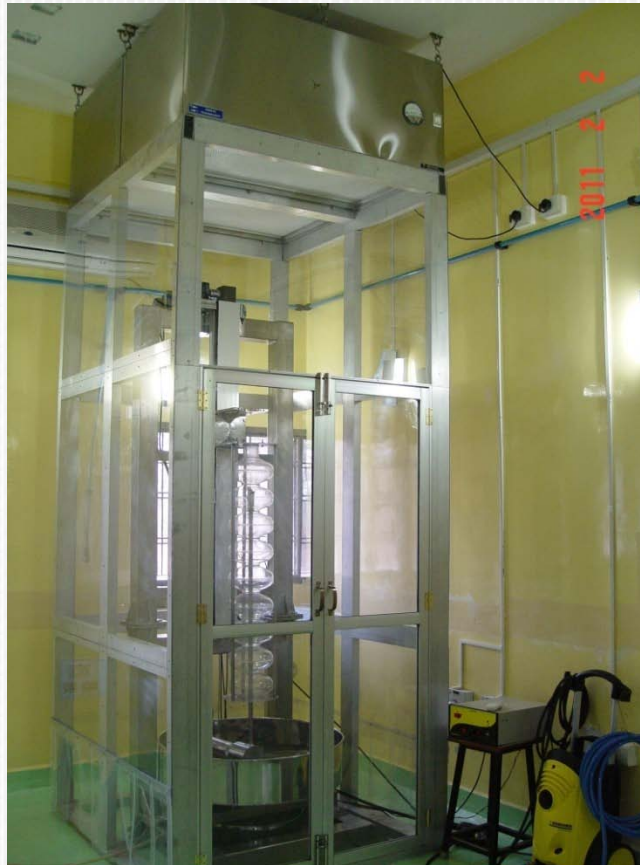
High Pressure Rinsing Set up in Clean enclosure (Class 100)
