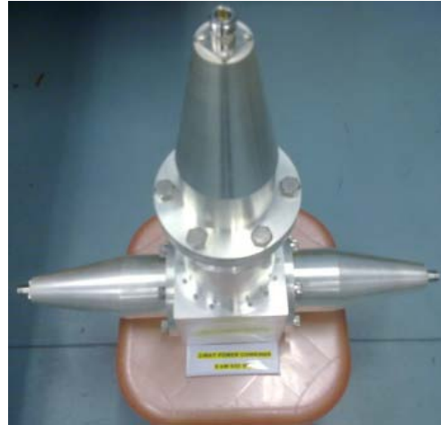
2-way 20 kW Power Combiner at 505.8 MHz
