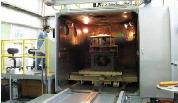
EB Welding at TOSEI co. Ltd.
