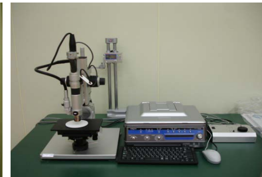
3D inspection equipment for Nb surface
